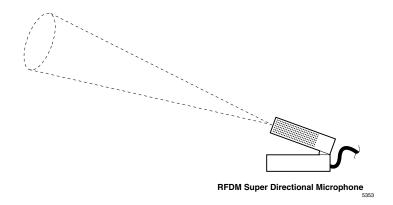
Figure 8 External Microphone Voice Pick-up Path
